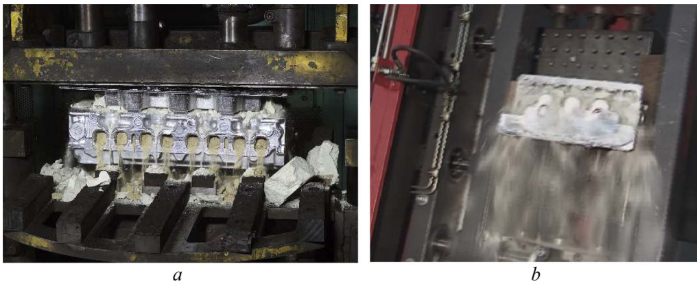
Fig. 1. Cylinder head with inorganic test cores during (a) hammering process and (b) shaking process (Nemak, 2005).
